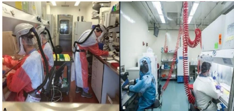
Fig. 7. Trained and authorised personnel's working in a BSL-4 laboratory wearing full-body positive pressure suit, fitted with air supplies (the positive pressure suit is completely attached with the personnel in A, while in B, it is attached with the facility) (Adapted from GERMFREE; USAMRIID). [39, 40]
