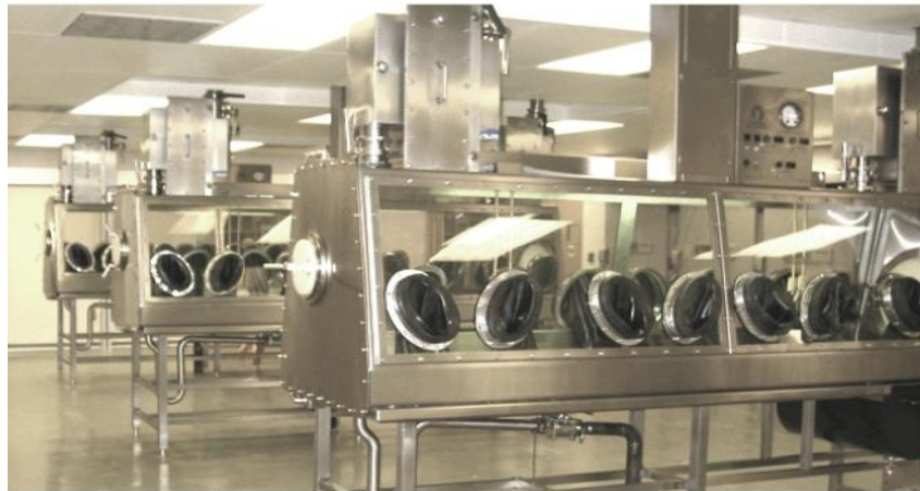
Fig. 6. BSL-3 and BSL-4 cabinet lab capabilities, fitted with gloves box lines and systems for All Hazard Receipt Facilities (AHRF) where samples must be handled at the highest levels of containment
